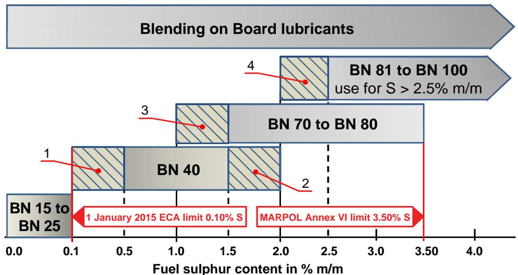
1. **0.1% < Sulphur < 0.5% m/m:** Inject cylinder oil at guide feed rate to prevent excess piston crown and top land deposits.
