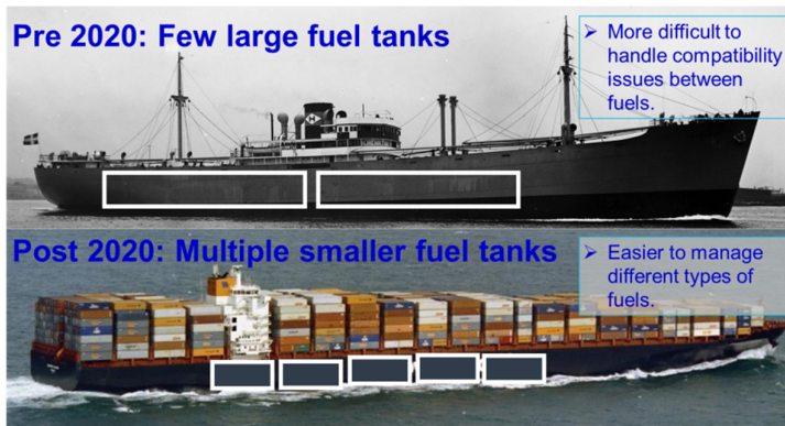
Figure 8 Before 2020: Ships were built with few, large tanks to ease the operation on board. After 2020: Ships should be built with multiple smaller fuel tanks to facilitate segregation of different fuel batches and decrease the risk of incompatibility between fuels.
