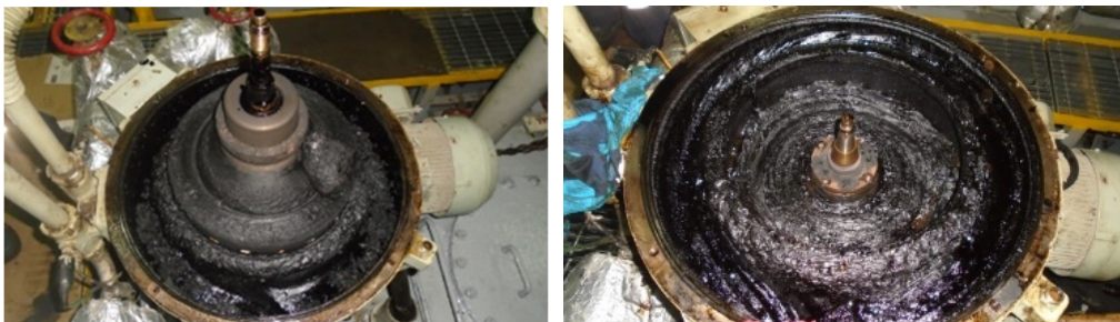
Figure 34 Heavy sludging and block separators as a result of either unstable fuel or incompatibility between two fuels.
