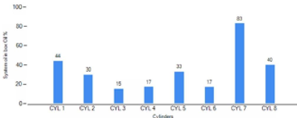
Example on Stuffing box performance by system oil leak rate per unit.
