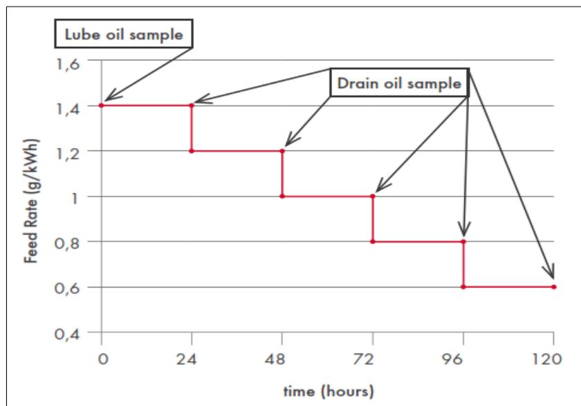
The sweep test procedure is very similar to the standard CSA sampling procedure:
