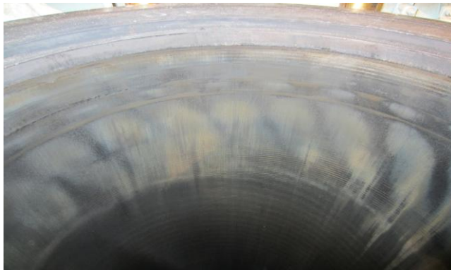
Fig. 1: Cold corrosion in upper part of cylinder liner
